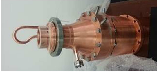
Fig. 1. (color online) The 60 kW coupler after fabrication.
