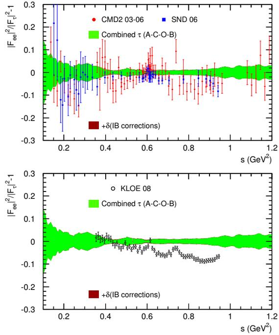
Fig. 4. Relative comparison between  $ee$  and  $\tau$  spectral functions, expressed in terms of the difference between neutral and charged pion form factors. Isospin-breaking corrections are applied to  $\tau$  data with the corresponding uncertainties included in the error band.
