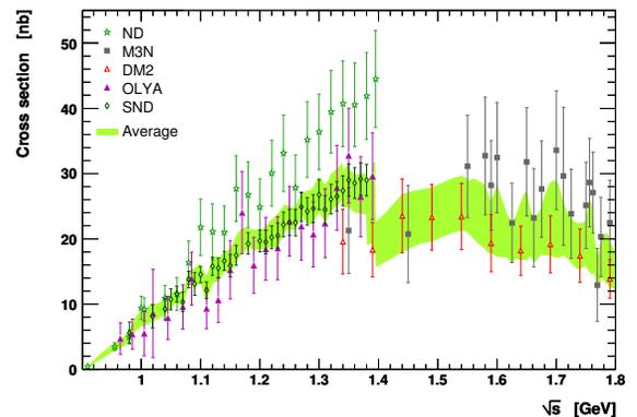
Fig. 8. Cross section measurements for  $e^+e^- \rightarrow \pi^+\pi^-2\pi^0$  used in the calculation of  $a_\mu^{\text{had,LO}}[\pi\pi 2\pi^0]$ . The shaded band depicts the HVPTools interpolated average within  $1\sigma$  errors. The individual measurements are referenced in Ref. [6].
